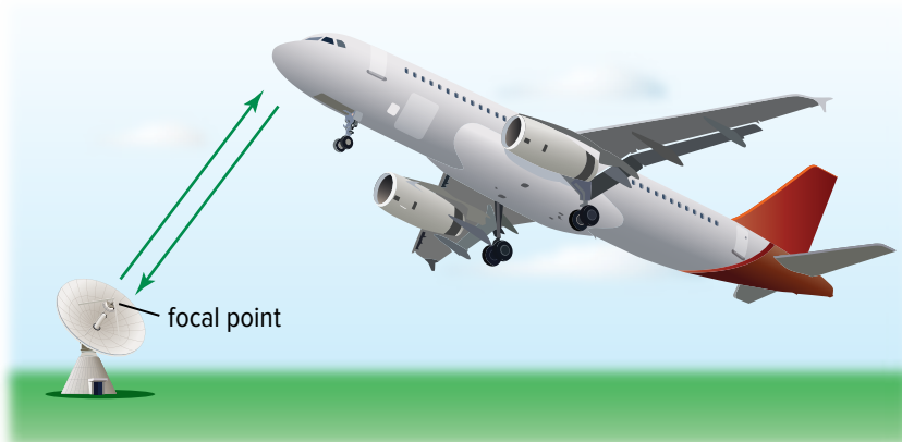
Figure 3.34 Concave and convex reflective surfaces both play a role in aircraft detection by radar.
