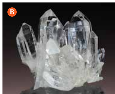
Figure 2.34 A Silicon dioxide, quartz, is a network solid. Its atoms are bonded into a regular, repeating structure by covalent bonds. This model shows a small part of the structure. In real quartz crystals like the ones shown in B , billions of atoms are bonded together in this same repeating structure, forming one giant molecule.
