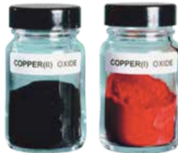
Figure 2.41: Although both of these compounds contain copper and oxygen, copper(II) oxide, \text{CuO} , is black and copper(I) oxide, \text{Cu}_2\text{O} , is red.
